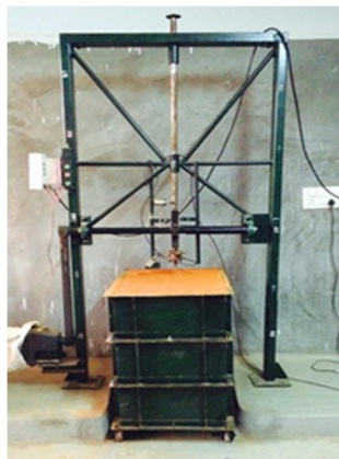
Figure 3: Test tank and loading frame (Courtesy: KSSEM Structures Lab)
